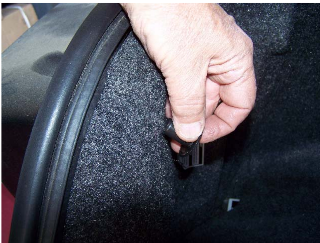
Unscrew and remove threaded plastic barrel fitting
