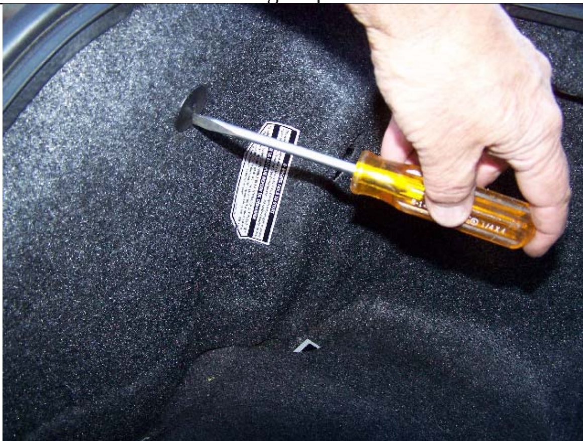
Open Trunk, and locate trunk liner retainer fitting
